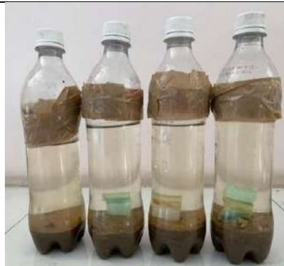
Figure 4: Winogradsky's column setup for plastic mask degradation
